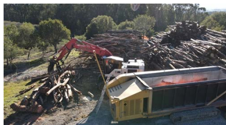
Pilot project at Anthony Chabot Regional Park using the carbonator to process onsite the biomass from the adjacent eucalyptus was completed in March 2023.
